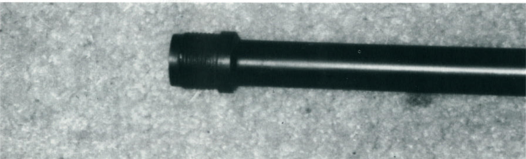
Muzzle end of barrel showing muzzle brake threads.
