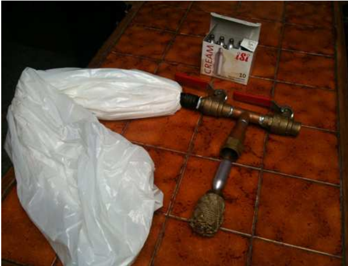
Figure 3.3. My nitrous wrench, with the storage bag on the left, mouthpiece on the right, a carton of nitrous cartridges above, and one cartridge shown ready to be screwed in at the bottom. The puncturing pin is in the bottom piece, which is covered with “needle hitching” (nautical rope work) for insulation from the cold due to the release of compressed gas.
