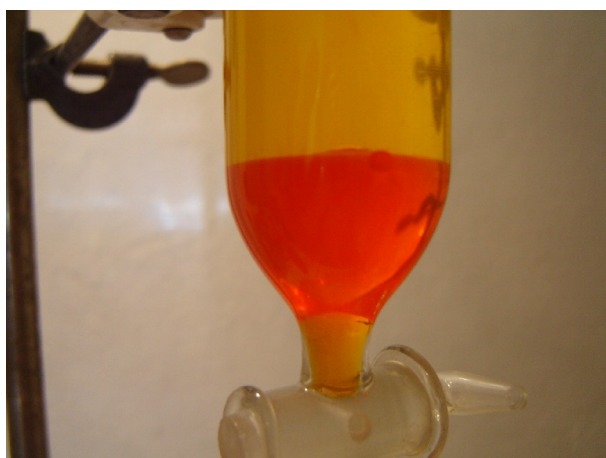
The DCM phase absorbing the bromine. an icebath, the freebase is first dissolved in the same volume of glacial acetic acid.
