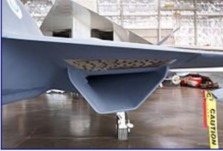
YF-23 [S-duct](#) engine air intake conceals engine from probing radar waves
