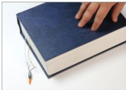
When the book is closed the circuit is off.
