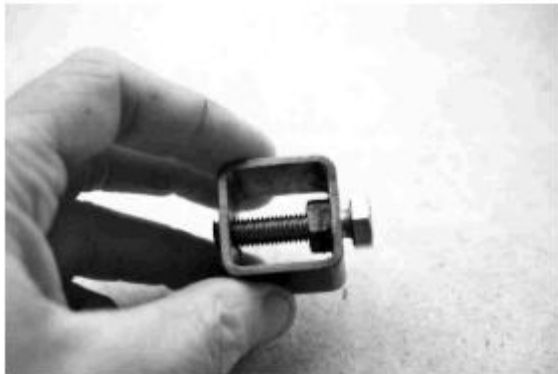
The finished die tool.
