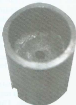
Place completed washer in breech piece (locked to barrel), with tin spacer separating washer and a round in the chamber. Weld washer fast to breech piece, maintaining headspace established by the empty round and tin spacer.
