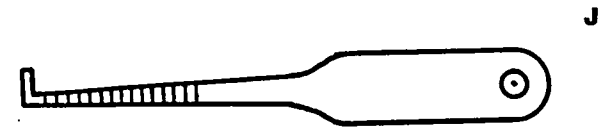
Figure 9C. With a carbide-tip tool engraver, meter your lock pick "J" for picking rotary tumbler locks. Etch lines .050" apart.
