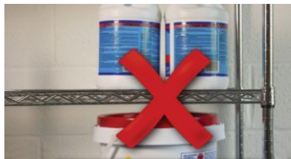
Figure 1. Never store liquids above dry chemicals
